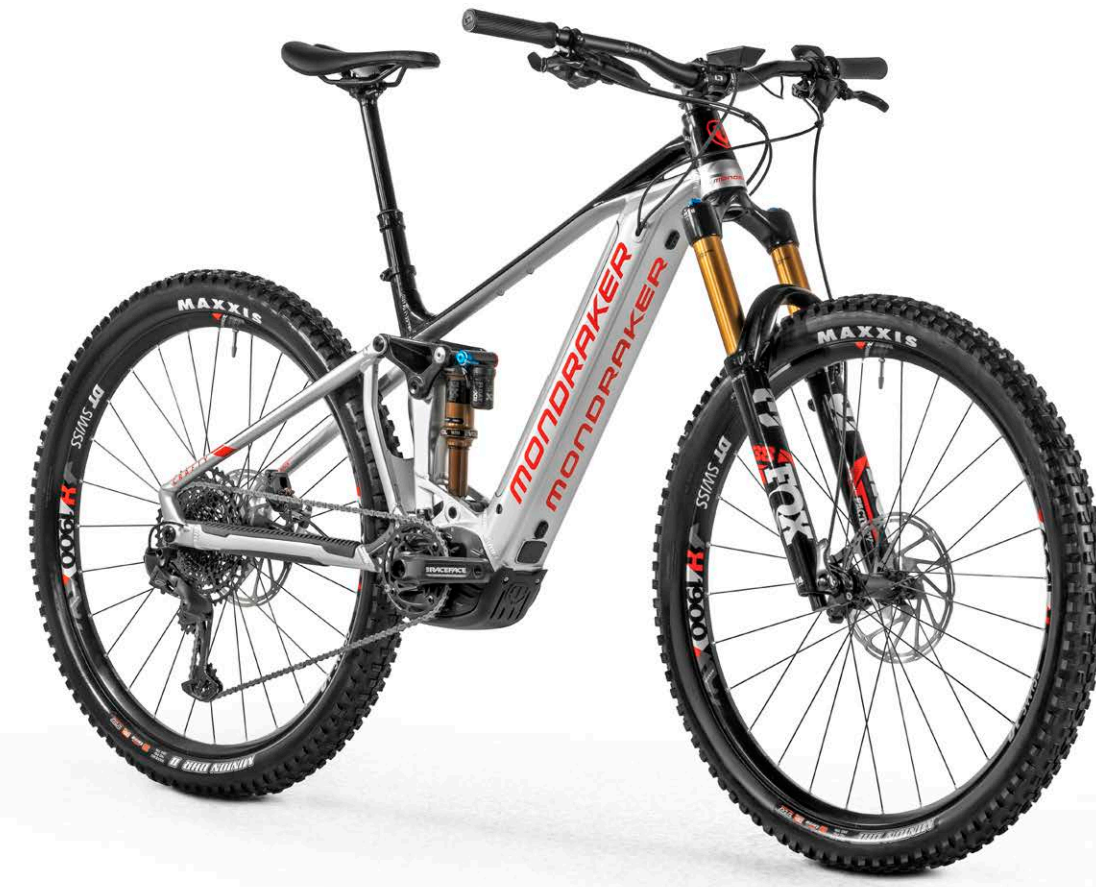
CRAFTY RR Stealth Alloy / Bosch Performance Line CX G4 / Bosch Powertube 625Wh / Fox Float DPX2 Factory / Fox Float 38 Factory / DT Hybrid H 1900 / Sram Code R / Sram GX Eagle
