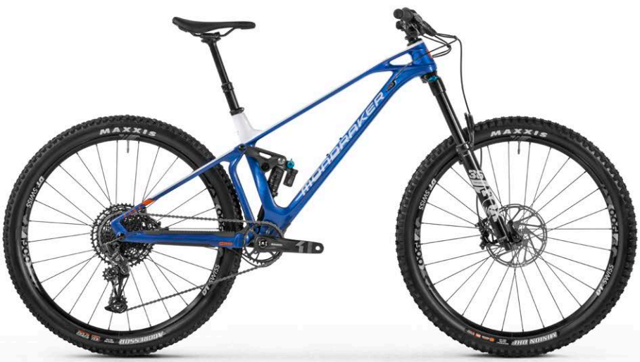
FOXY CARBON R Stealth Air Carbon / Fox DPX2 Performance / Fox Float 36 Performance / DT E1900 / Sram G2 R / Sram NX Eagle
