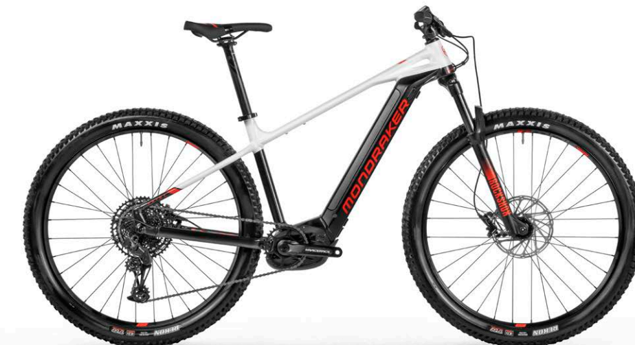
PRIME / COLOR 1 Xtralite Alloy / Bosch Performance Line CX G4 / Bosch Powertube 625Wh / RockShox Recon Silver RL / MDK-HP1 TL30 ASY / Sram Level T / Sram SX Eagle
