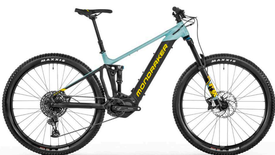
DUSK R Stealth Alloy / Shimano EP8 / Simplo 630Wh / Optional Simplo 360Wh range extender / Fox Float DPS Performance / Fox Float 36 Rhythm / MDK-HP1 TL30 ASY / Sram G2 R / Sram SX Eagle / Onoff Pija
