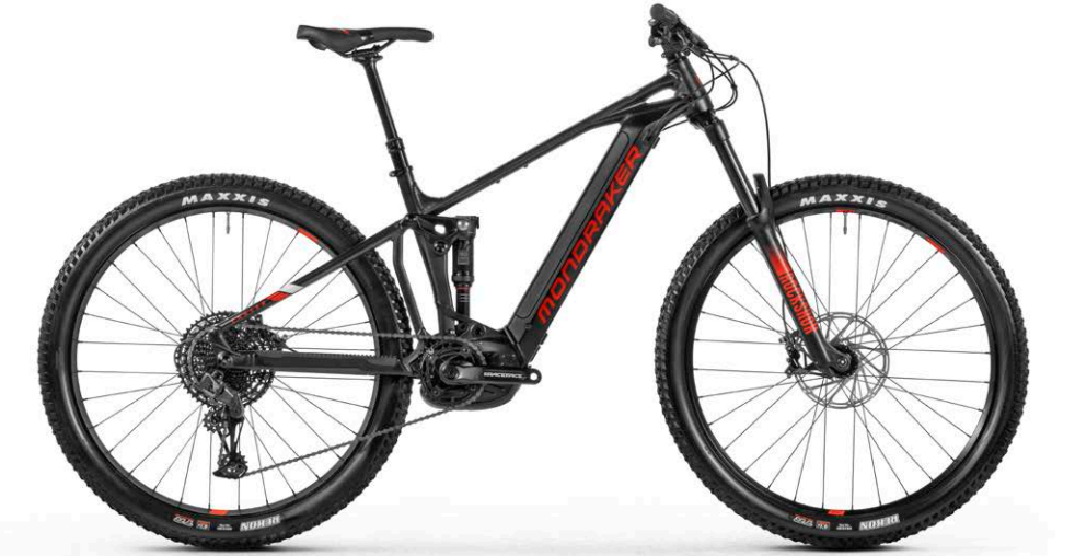
CHASER / COLOR 1 Stealth Alloy / Bosch Performance Line CX G4 / Bosch Powertube 625Wh / RockShox Deluxe Select R / RockShox 35 Silver TK / Sram G2 R / Sram SX Eagle / Onoff Pija
