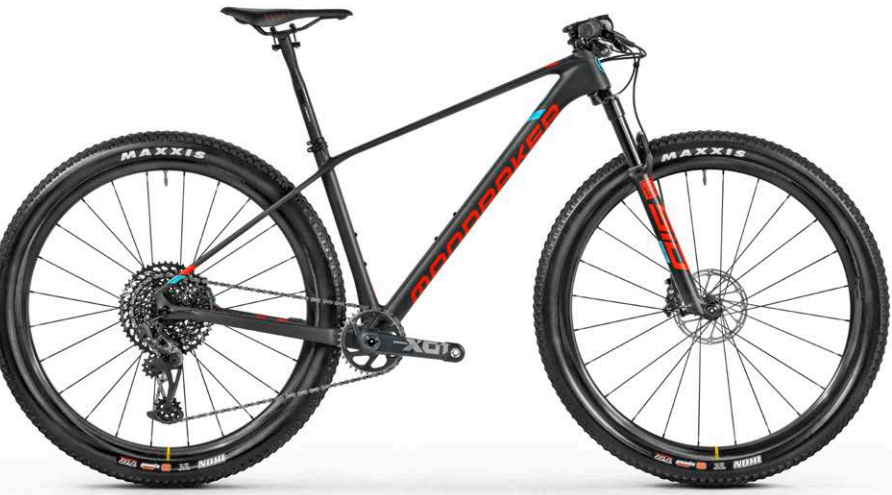
PODIUM RR Stealth Air Carbon / RockShox SID SL Ultimate / Mavic CrossMax Carbon SLR / Sram Level TLM / Sram X01/GX Eagle
