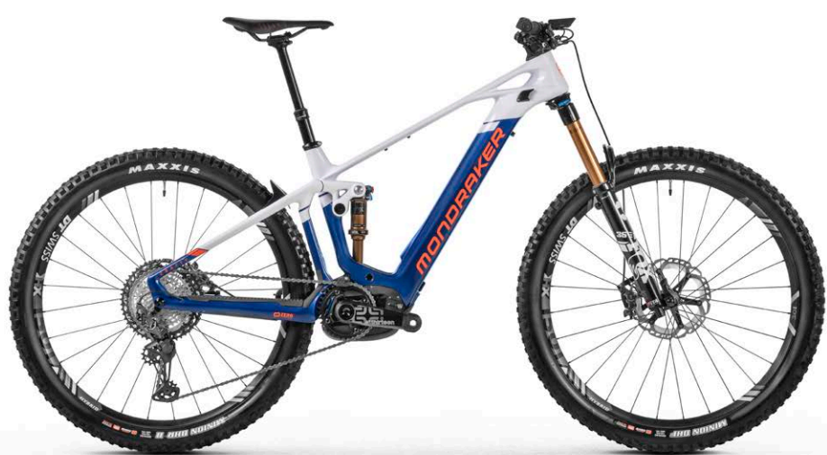
CRAFTY CARBON RR Stealth Air Carbon / Bosch Performance Line CX G4 / Bosch Powertube 625Wh / Fox Float DPS Factory / Fox Float 36 Factory / DT Hybrid HX 1501 / Sram G2 RSC / Sram X01/GX Eagle
