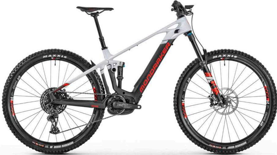
CRAFTY CARBON R Stealth Air Carbon / Bosch Performance Line CX G4 / Bosch Powertube 625Wh / Fox Float DPS Performance / Fox Float 36 Performance / DT Hybrid H 1900 / Sram G2 RSC / Sram GX/NX Eagle
