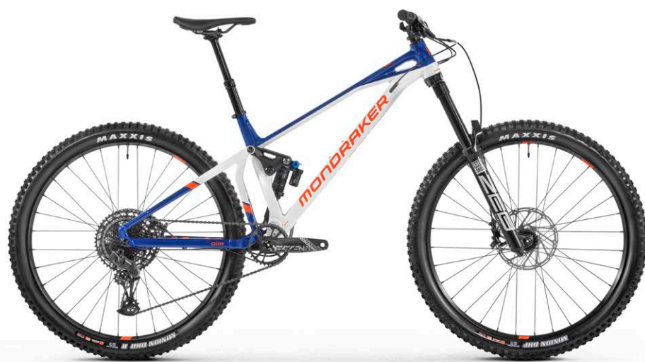
SUPERFOXY Stealth Alloy / Fox Float DPX2 Performance / RockShox ZEB Select RC / MDK-EPI TL30 ASV / Sram G2 / Sram SX Eagle
