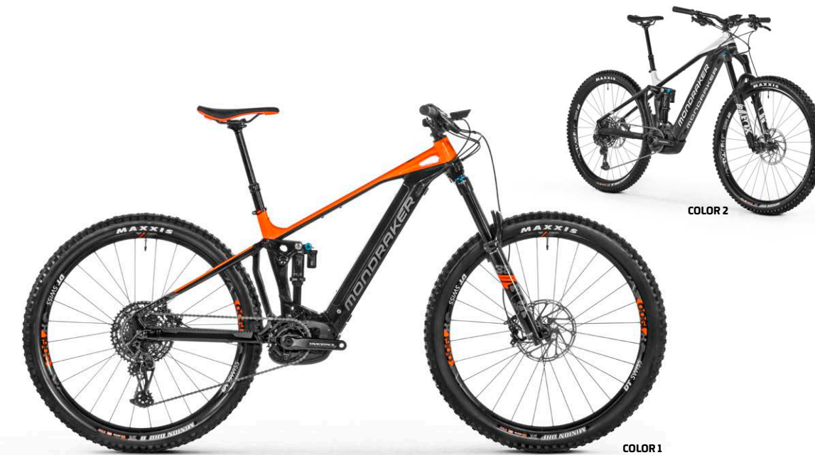
CRAFTY R Stealth Alloy / Bosch Performance Line CX G4 / Bosch Powertube 625Wh / Fox Float DPX2 Performance / Fox Float 38 Performance / DT Hybrid H 1900 / New Sram G2 R / Sram GX/NX Eagle
