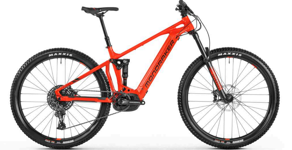
CHASER / COLOR 2 Stealth Alloy / Bosch Performance Line CX G4 / Bosch Powertube 625Wh / RockShox Deluxe Select R / RockShox 35 Silver TK / Sram G2 R / Sram SX Eagle / Onoff Pija
