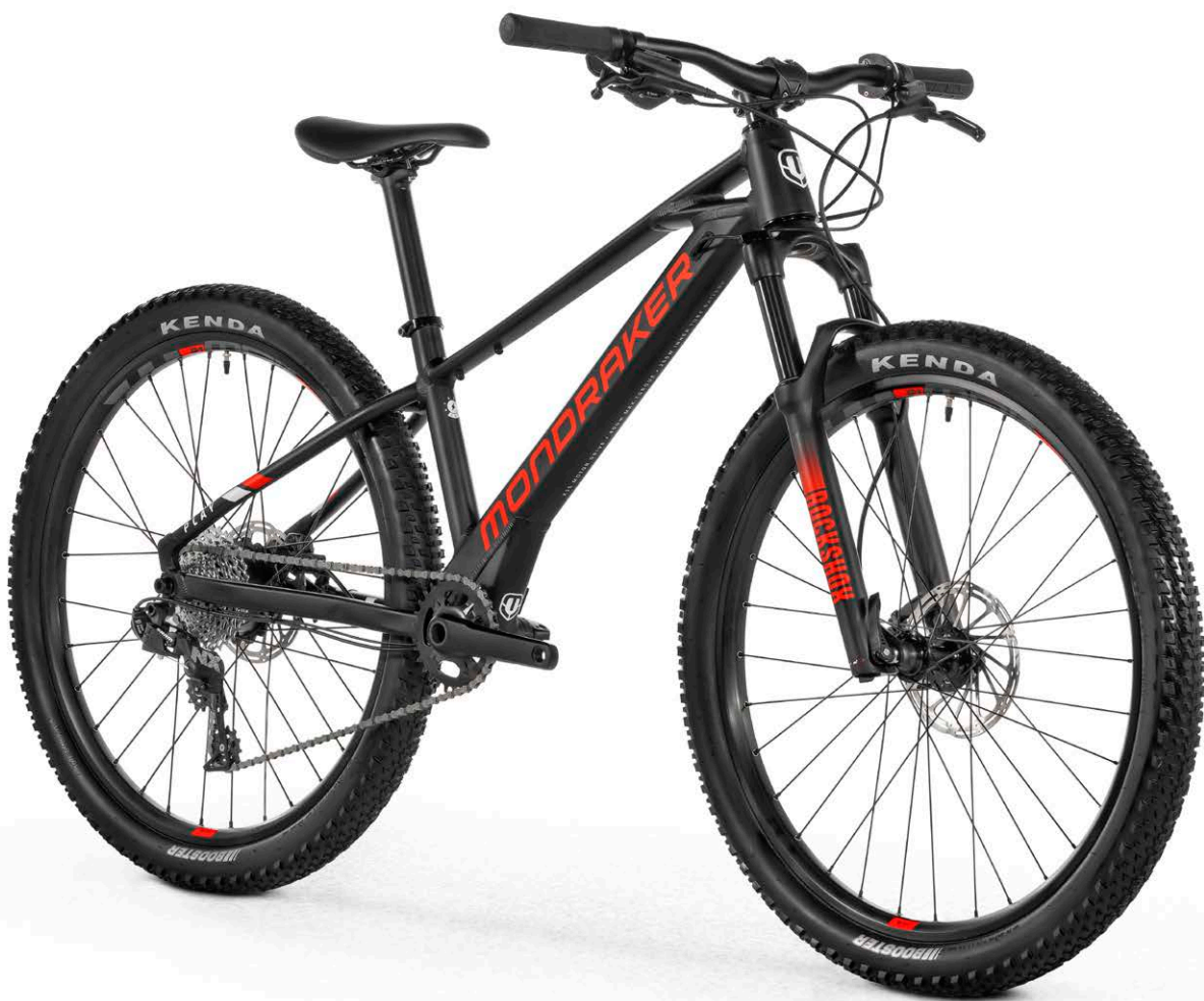
PLAY 26 Stealth Alloy / Mahle e-Bikemotion X35 / 250Wh battery / RockShox Judy Silver TK / Sram Level / Sram NX 11s
