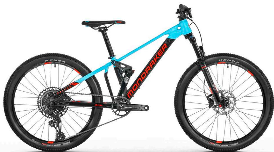
FACTOR 24 Stealth Alloy / X-Fusion Q2Pro R / X-Fusion Velvet RL / Shimano M4100 / Sram SX Eagle
