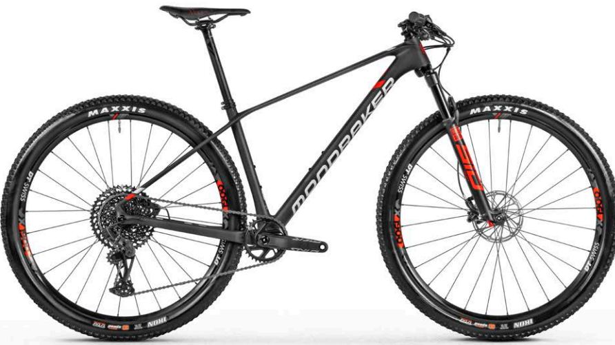
PODIUM Stealth Air Carbon / RockShox SID SL Select / DT Swiss X1900 / Sram Level TL / Sram GX/NX Eagle
