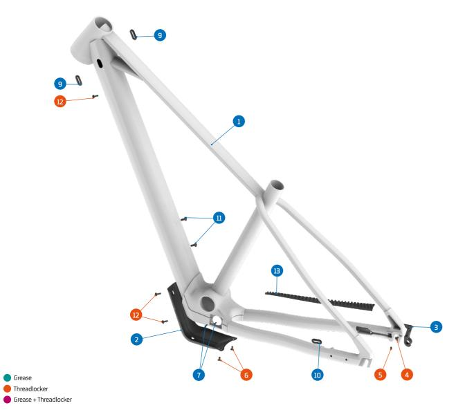
Apply grease to the shaft, and locker to the threads
